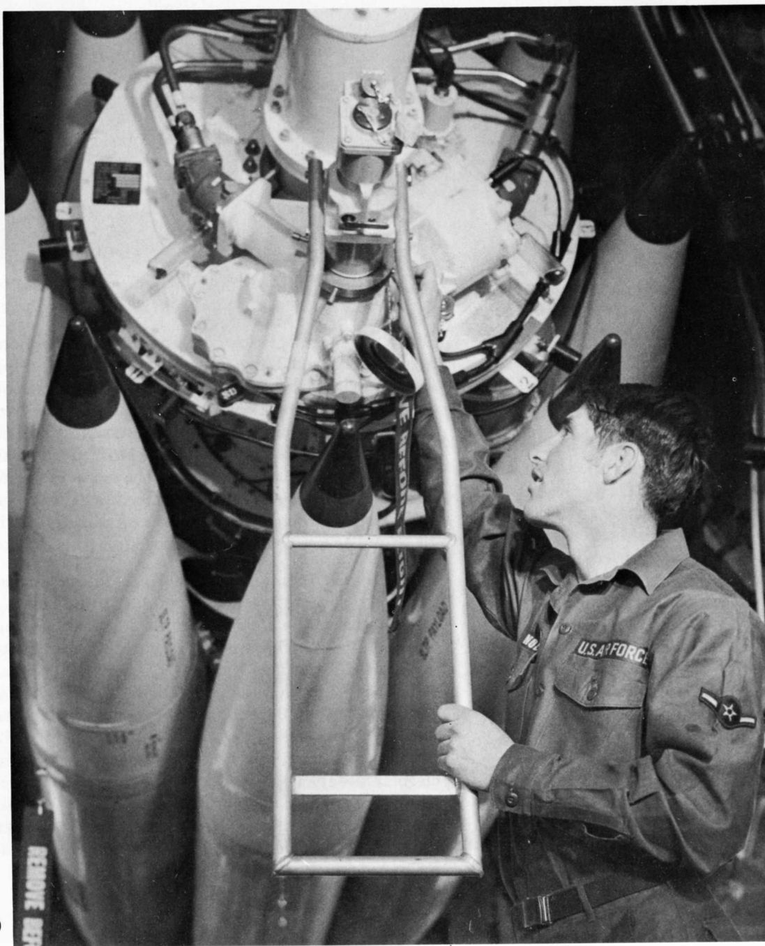
This munitions student is training on the SRAM rotary launcher for the B-52 aircraft.
