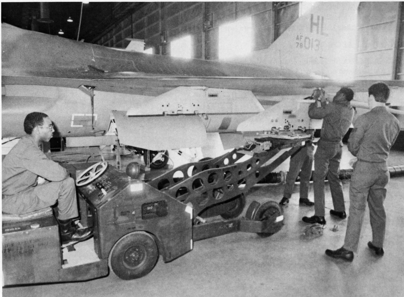
Since 1980, Lowry has prepared avionics and armament specialists for the F-16 aircraft. These students are attaching wing pylons.
