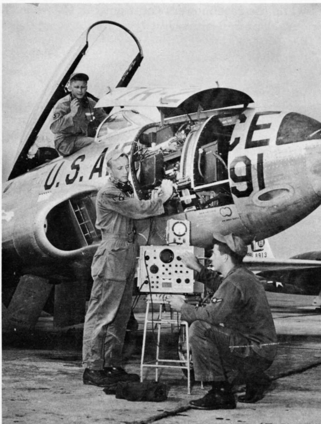
Technicians from Lowry's 3415th Maintenance and Supply Group check the electronic systems of a T-33 aircraft.
