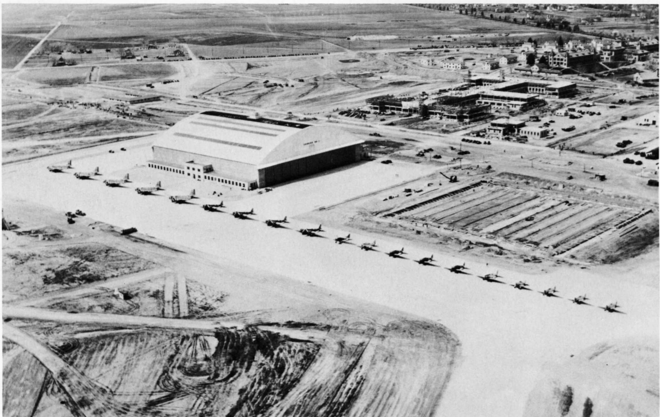
In December 1939, Lowry's flying heritage began in earnest when the aircraft assigned to the post were ferried from their temporary location at Denver Municipal Airport. This 1940 photograph of the flight line shows five Douglas B-18s, four Martin B-10s, and several single-engine aircraft, including a Seversky P-35 and some Curtiss P-36s.
