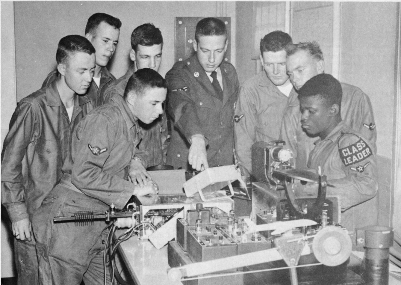
A class in the Department of Fire Control Systems Training receives instruction on test equipment for the AN/APQ-30 gun-sight used on the F-102 aircraft.
