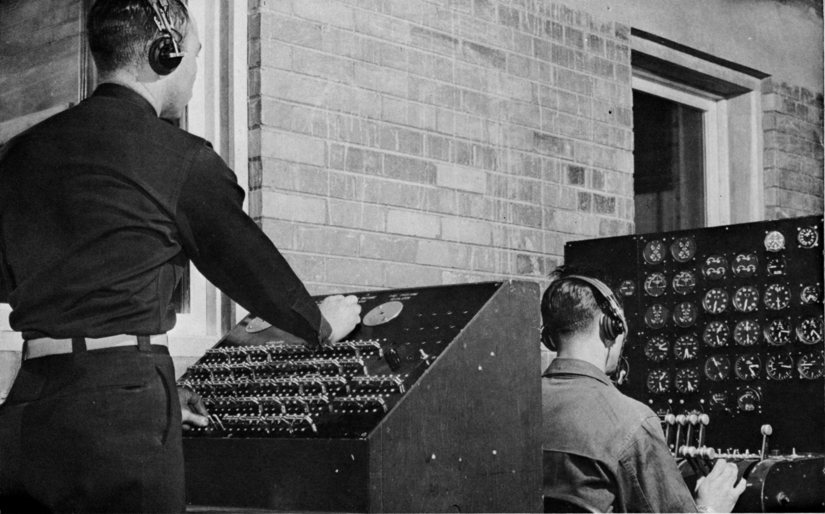
In October 1943 the Army transferred the Flight Engineers School to Lowry. This 1945 photograph shows a B-29 flight engineer station and trainer.
