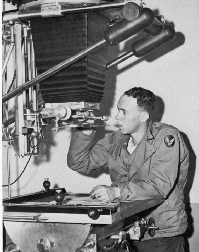
Photography students used the B-9 projection printer to prepare aerial photographs, (Frank Mouffe)
