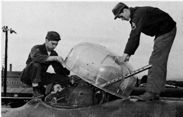
The Martin upper turret being inspected by these students was installed on B-24 and B-26 bombers.
