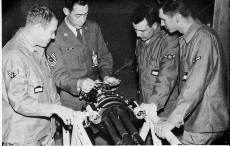
The M-61 Vulcan gun was installed on F-104, F-105, and F-111 aircraft. The M-61 fired up to 6,000 rounds of 20 millimeter ammunition per minute. Lowry began M-61 instruction in the late 1950s.
