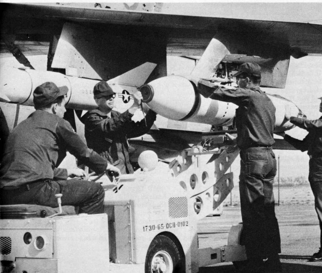
Students in the Department of Aerospace Munitions Training load a cluster bomb on an F-105.
